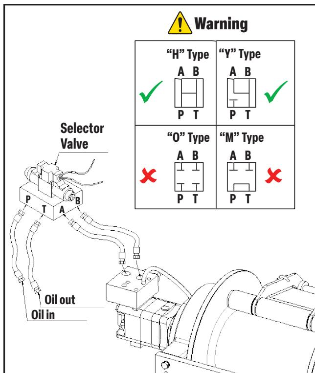
Hydraulic control valves are an essential component for optimizing system performance. They're used to regulate the flow rate and pressure of the hydraulic oil as it passes through a hoses or pipes, always maintaining the speed and pressure.
